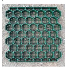
The support base and the rings' walls prevent soil compaction and reduce rutting and erosion by supporting the weight of traffic and concentrated loads, while the large void spaces in the rings allow a strong root network to develop. The end result is a load-bearing surface covered with natural grass and which is typically around 90% pervious, allowing for stormwater pollution filtration and treatment.
